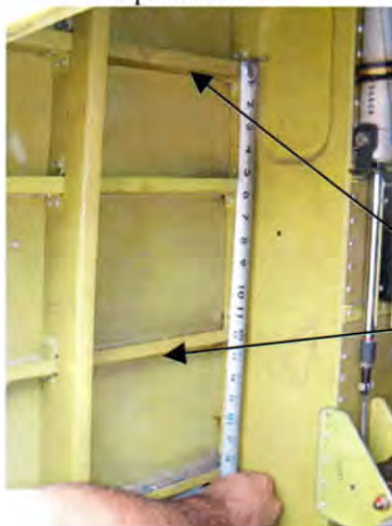
Template C transfer to bottom side of these stringers
