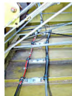
View from tail - left access Fuel line and electrical secured as described in fig 2. A-A & B-B.
