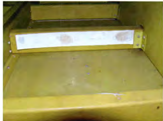
Template C transfer to bottom side of these stringers
