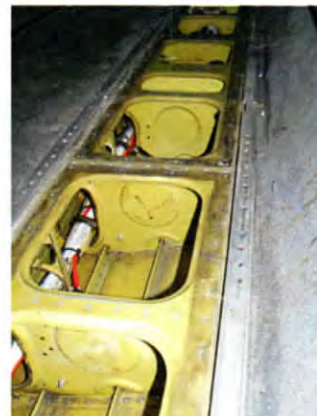
Existing wire bundle looking forward
