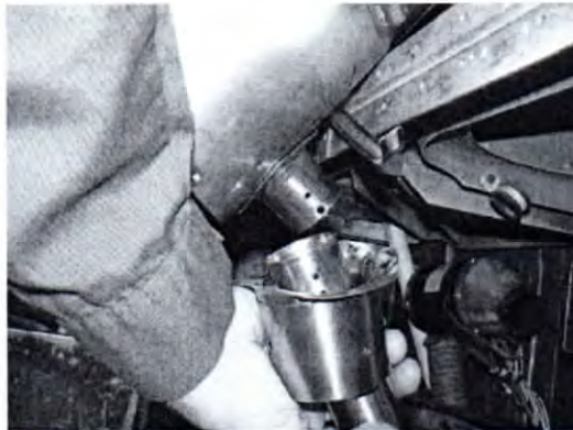
First noting orientation, remove 4 screws holding exhaust shroud to heater jacket. And 2 screws holding exhaust extension to combustion tube.
